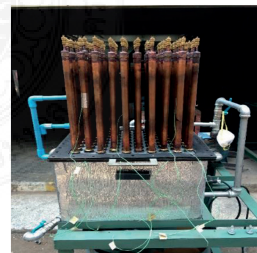
Fig. 2 Design of the experimental thermosy-phon showing schematic layout (upper), actual test unit (middle) and thermosyphon heat exchanger (lower)
