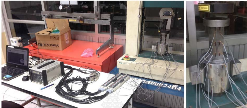
Fig. 3 Strain gages installation on upper punch and waveguide
