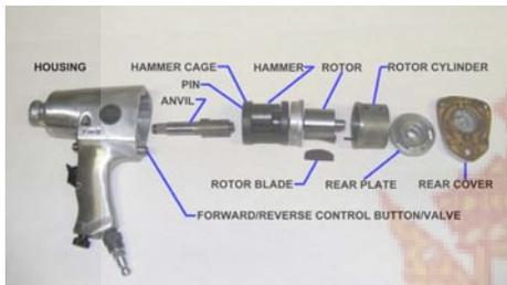
Fig. 3 Parts of impact wrench [1]
