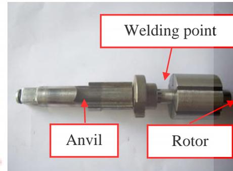
Fig. 4 Impact wrench parts before welding
