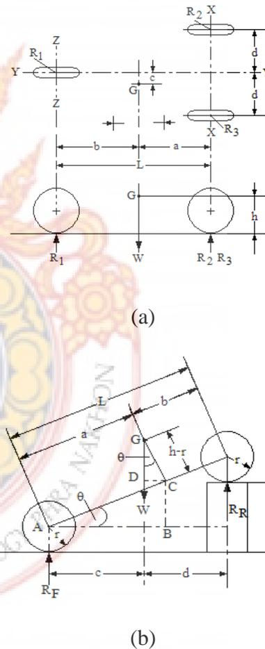
Fig. 7 Dimensions of car and reaction forces on wheels
