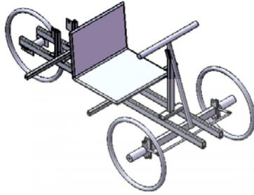
Fig. 9 Air car structure
