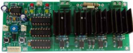
Fig. 5 Driver motor board
