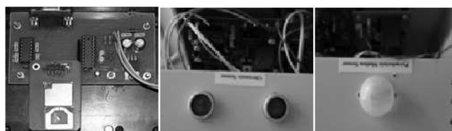
Fig. 7. The transducers with the indicators and the transceiver modules
