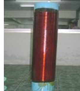
Figure 3. High voltage binding with 6 inch. PVC tube
